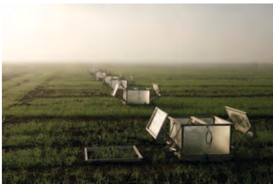
Greenhouse gas emissions being measured using a fully automated system. These measurements will be used in the development of methodologies under the Carbon Farming Initiative.
